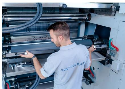
New doctor blade chamber with innovative design by Koenig & Bauer Flexotecnica
