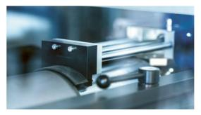
Pneumatic ejectors for quick and simple printing and anilox sleeve removal in utmost safety by avoiding scratches or damage, particularly with wide printing widths and large print repeats
