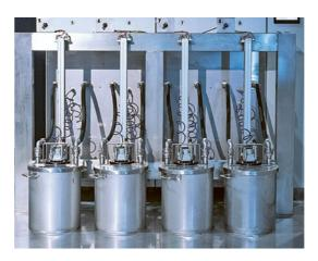
**"WashTronic" automatic washing system** with digital control of all washing cycles via the touchscreen for both solvent and water based inks. The system ensures all inking groups on all print units are washed simultaneously in only a few minutes — or only those selected by the operator — and with minimized consumption of solvent or water.
