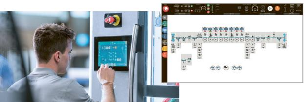
**ErgoTronic** is the name of the new control system for Koenig & Bauer Flexotecnica printing presses featuring completely new PLCs, motion logic drives and high quality industrial operator panels to achieve increased system performance, accuracy and reliability.
